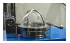
The main component of this machine, so designed as to withstand high vacuum, as well as to attain vacuum by merely closing the lid without any clamping required. The upper side of the chamber has a glass dome. The chamber is tested upto  $5 \times 10$ -6 Torr.
