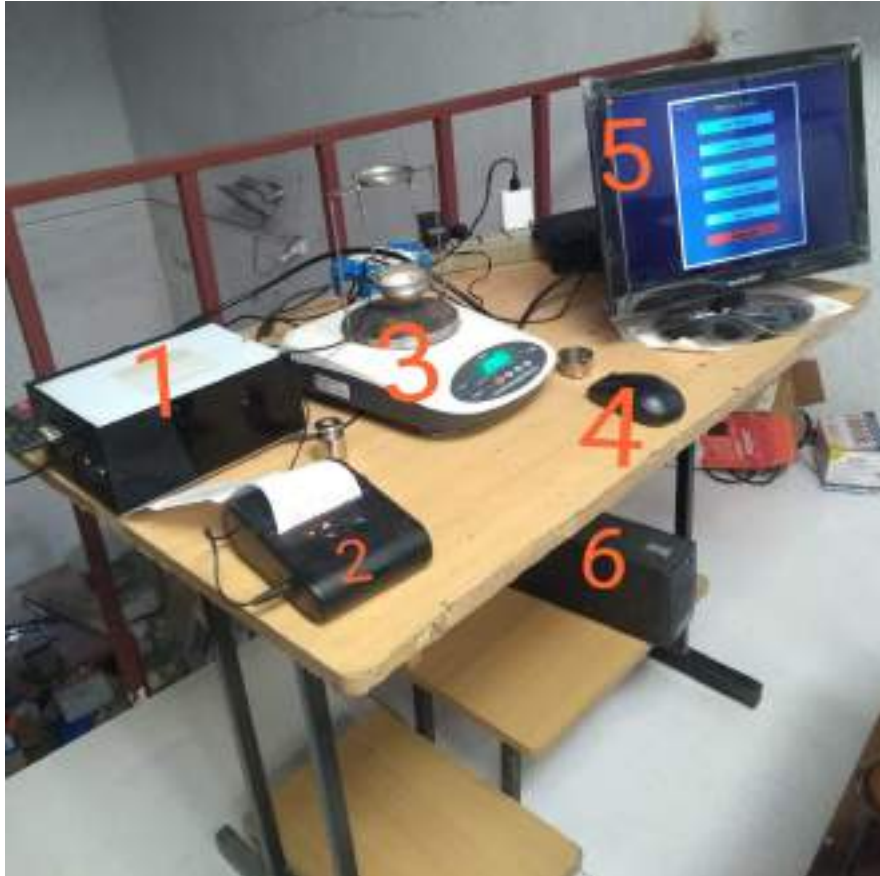
1. Hardware with programmed software. 2. Thermal printer. 3. High precision weighing machine 4. Wireless mouse (keyboard not visible in picture). 5. 18" monitor. 6. UPS
